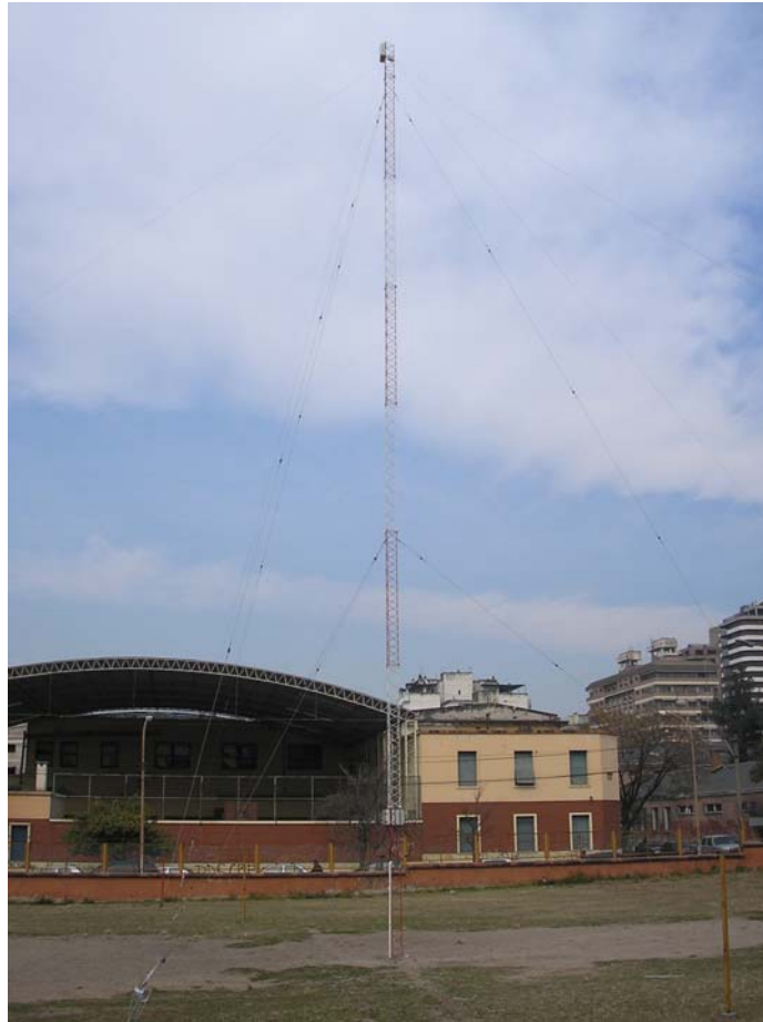
Figure 2. The delta antenna of the new ionospheric station of San Miguel de Tucumán.
