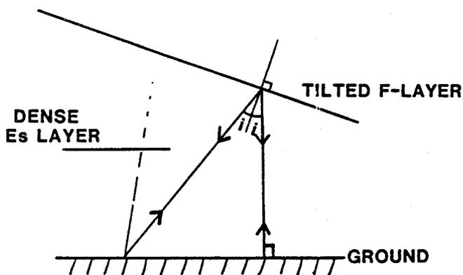
Fig. 3 Schematic illustration showing another method under which the first order traces from the F layer are missing but a second order type trace is seen.
