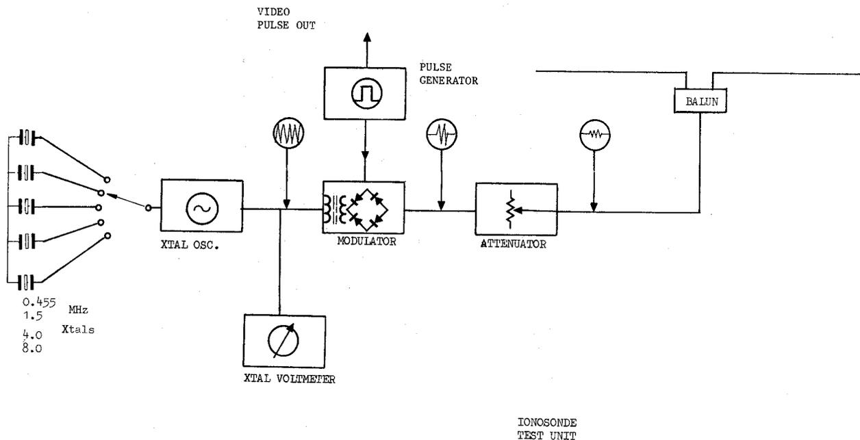
A crystal oscillator (XTAL OSC) contains a set of crystals one for each band of the ionosonde, plus an extra position for another spot frequency. The c.w. signal is monitored by a crystal voltmeter and converted to radio frequency pulses of measured amplitude in the modulator.
