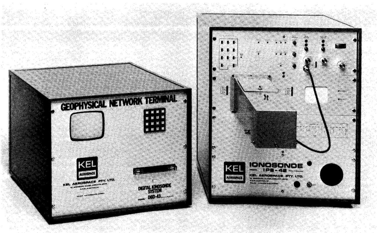
The KEL Aerospace DBD-43 Digital Add-On System for the IPS-42 ionosonde is a design which has evolved over the last four years following the design concept of the original DBD-42 and the many design changes and technical improvements that resulted from that initial project.
